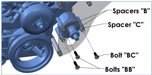
Front bracket shown transparent for better visualization of spacer placement.
