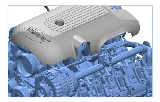
3. Remove the main accessory belt by rotating tensioner clockwise.
