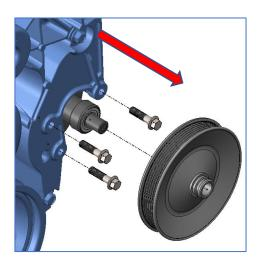
7. Remove the four mounting bolts from the factory bracket.
